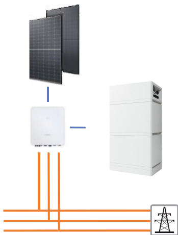
Single- or Three-Phase Connection with Hybrid Inverter
