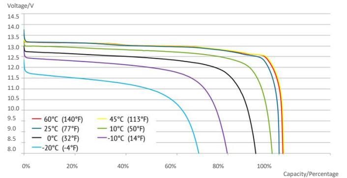
Discharge voltage Characteristic at different Temperature
